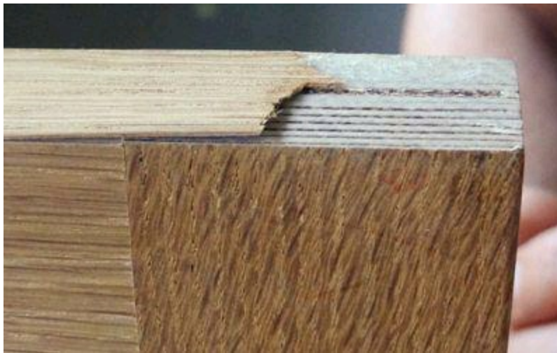
Torn and missing veneer
