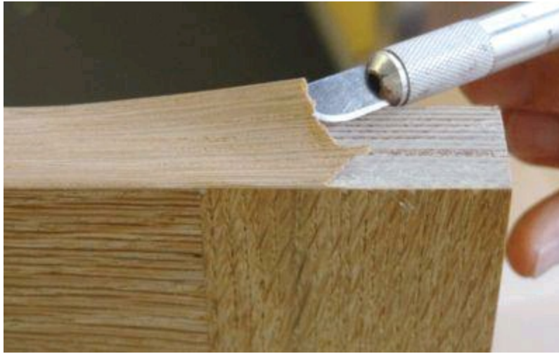
Lifting and unglued veneer
