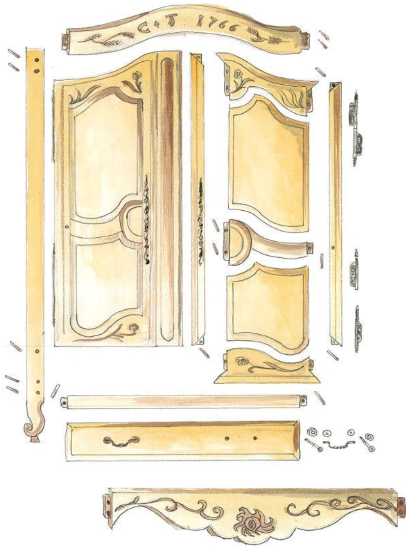
The front, dismantled: Construction is all mortise-and-tenon, with wood pegs that allow pieces to expand and contract in response to weather and environmental conditions.
